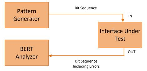
Although a PRBS sequence demonstrates random behaviour, it's in fact generated deterministically and the bit sequence will always be the same when repeated. As an example, a PRBS7 sequence has a word length of 7-bits and will generate a sequence length of 2^7-1(127) bits, which is repeated indefinitely by the pattern generator. In general, any PRBSk sequence will have a word length of k bits and a sequence length 2^k-1 bits. It's this combination of both deterministic generation and random bit
