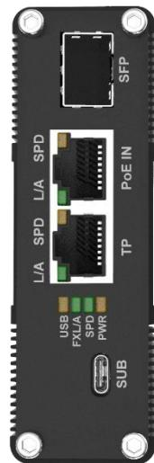
The FR-IPM2003MT Series is an advanced industrial PoE-to-Fiber transceiver. It features IEEE 802.3at/bt power input and uniquely provides a 60W USB-C PD output to charge modern devices. It offers one 10/100/1000BASE-T RJ45 port and one 100/1000BASE-X SFP port, effectively bridging copper and fiber networks for long-distance data extension.
